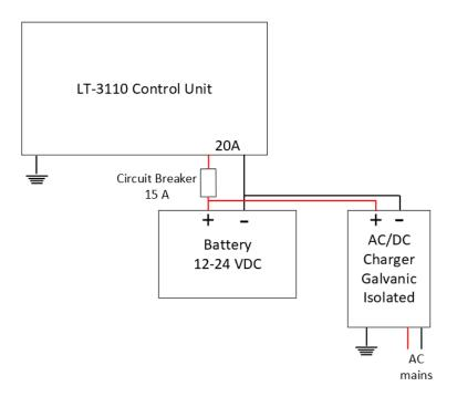
Figure 57: Battery Power Supply
