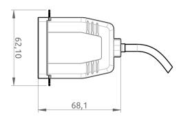
Figure 372: Outline Drawing: LT-3160S Printer Adapter
