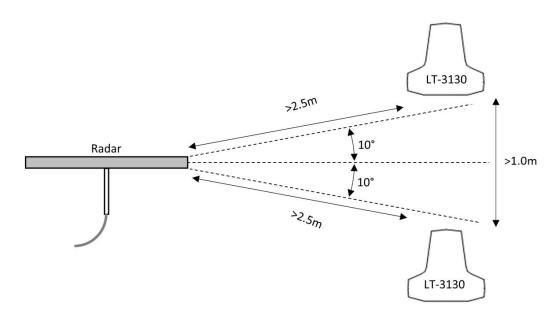
Figure 13: LT-3130 Antenna Unit (avoid the radar beam)
