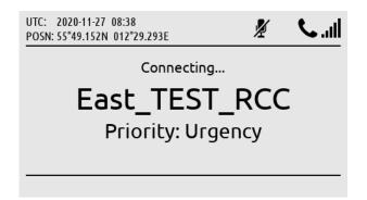
The Safety Call is connecting to the RCC (in this example East\_TEST\_RCC).
