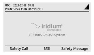
LT-3110S Control Unit, default window. A Safety Message can be initiated by pressing the soft key 'Safety Message'.
