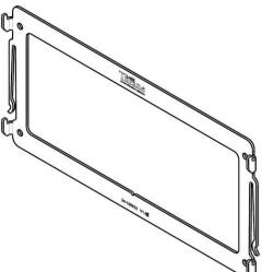
Figure 4: Bracket Mount, Control Unit.
