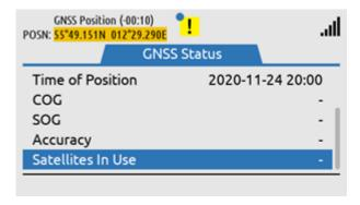
Figure 361: GNSS Receiver Integrity State
