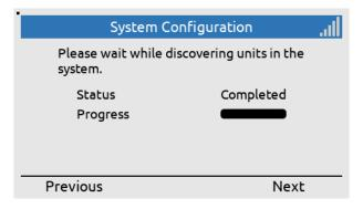
The LT-3110S CU is searching for LT-3100S GMDSS system units part of the setup.
