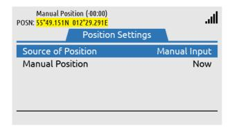
Manual Position is now being used as the position in the system. See information in the status bar (position is colored yellow to indicate low integrity).
