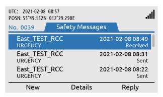
After the Safety Message has been opened (and read) the unread symbol and BAM alert will be removed.
