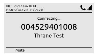
Use the off-hook button, # key, or wait 10 seconds for the LT-3100S GMDSS system to start connecting the voice call.
