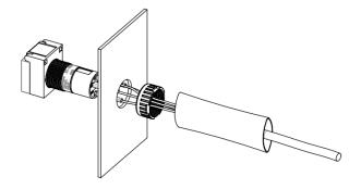
Figure 26: Install SSAS Alert & SSAS Test button (1 of 3)
