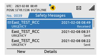
Read the Safety Message by pressing the ENTER button or use the soft key 'Details'.
