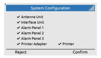
The LT-3110S CU has identified the following LT-3100S GMDSS system units, confirm to continue.
