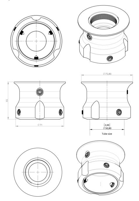
Figure 374: Outline Drawing: Pole Mount (2.0" pipe, Ø53.0 mm), Antenna Unit
