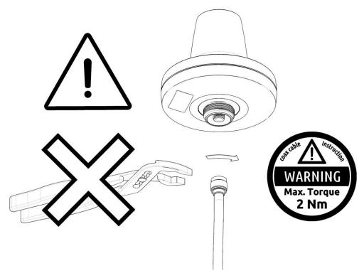
Figure 11: Connecting the coaxial cable N connector to the LT-3130 Antenna Unit
