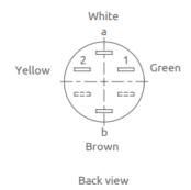
Figure 51: SSAS Test button (back)
