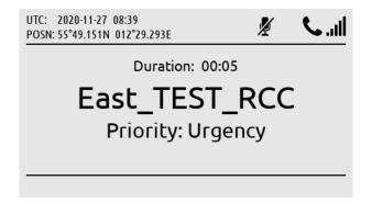
The Safety Call is connected (duration counter will start to count when the RCC has been connected).
