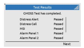
The results of the system verification are listed in the Test Results screen Test Results (Top view)
