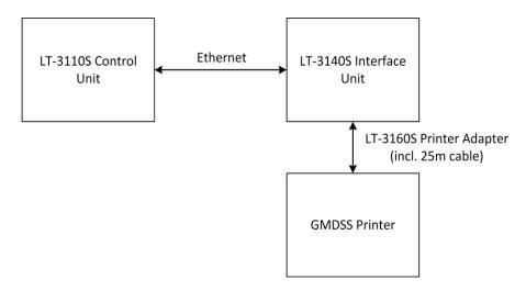
Figure 305: Connect a GMDSS Printer
