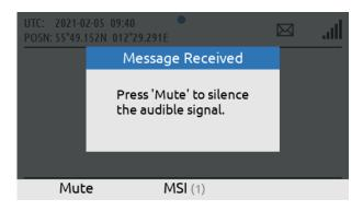
The LT-3100S GMDSS System has received a new MSI message with priority of Urgency or Distress. The audible alarm can be muted by pressing 'Mute'
