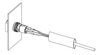
Figure 27: Install SSAS Alert and Test button (2 of 3)
