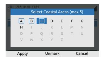
On-going marking of the Costal Warning Areas to be added. Use the soft key 'Apply' when completed.
