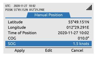
SOG must be entered. Use soft key 'Apply' when all inputs have been entered correctly.
