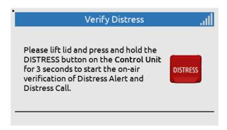
Lift the lid and press the DISTRESS button on the LT-3110S Control Unit.
