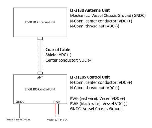
Figure 54: Definitions of VDC (+), VDC (-), and GNDC
