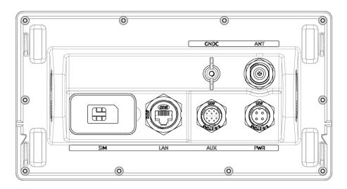
Figure 3: LT-3110S Control Unit (back view)
