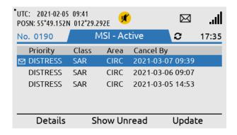
The MSI message is a Distress Alert Relay message, Class SAR (Search and Rescue). The MSI message can be read by pressing the soft key 'Details'.
