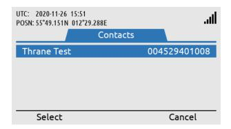
If Contacts has been chosen, then select the contact by using the Navigation key and the soft key 'Select'.
