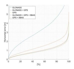
Figure 342: GNSS receiver horizontal position error
