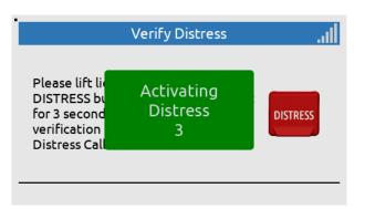
The DISTRESS button must be held for a minimum of 3 seconds to activate a Distress.
