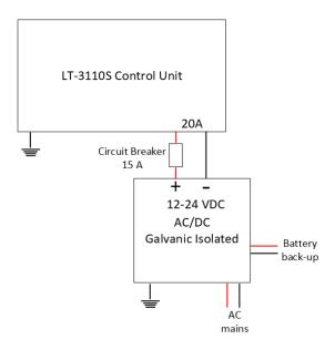
Figure 55: AC/DC Galvanic Isolated Power Supply
