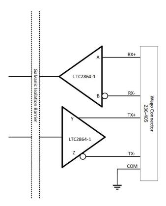
Figure 43: RS-422 Circuit Diagram for the LT-3140S IU
