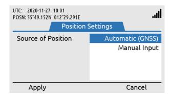
Source of Position is changed from Automatic (GNSS) to Manual Input. Use the soft key 'Apply'.
