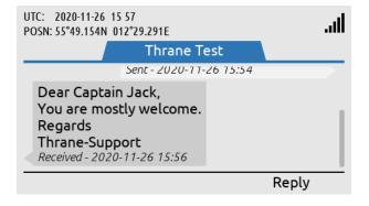
Use the ENTER button to open the received SMS.
