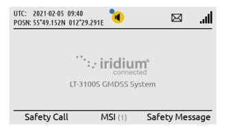
By pressing 'Mute' the system returns to the default screen. The BAM alert symbol and MSI(1) indicates that the priority message has not yet been read.
