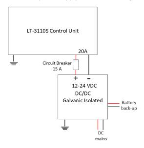
Figure 56: DC/DC Galvanic Isolated Power Supply
