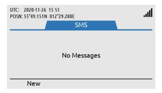
No SMS' are available in the LT-3100S GMDSS system (sent or received). Use soft 'New' to prepare a new SMS.
