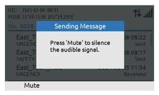
Sending a Safety Message of Urgency priority generates an audible alert. Press the soft key 'Mute' to mute the audible alert
