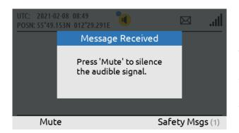
Receiving a Safety Message of Urgency or Distress priority generates an audible alert. Press the soft key 'Mute' to mute the audible alert
