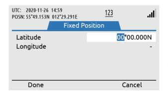
Inserting position (latitude and longitude) in order to receive MSI information from this point of interest.
