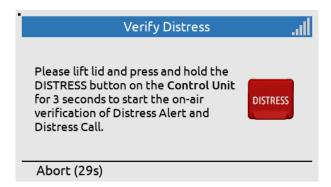
The DISTRESS button on the LT-3110S Control Unit must be used to activate the Terminal Test.
