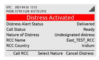
Call Status = Ready (Distress Call has been disconnected to the RCC). Use soft key 'Call RCC' to activate a new Distress Call.
