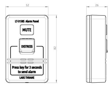
Figure 371: Outline Drawing: LT-3150S Alarm Panel
