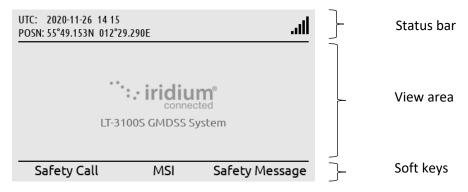
Figure 59: LT-3110S Control Unit (display sections)
