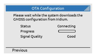
The LT-3100S GMDSS system is down-loading the GMDSS Configuration file (connecting).
