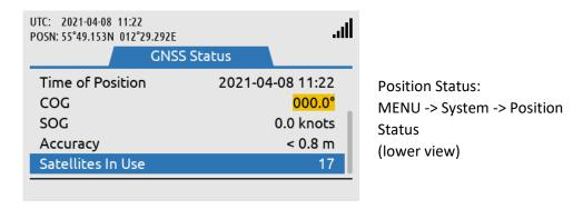
Figure 287: System submenu (Position Status)
