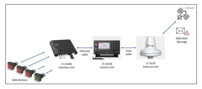
Figure 306: SSAS System Setup (end-to-end)
