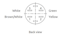
Figure 44: SSAS Alert button (back)
