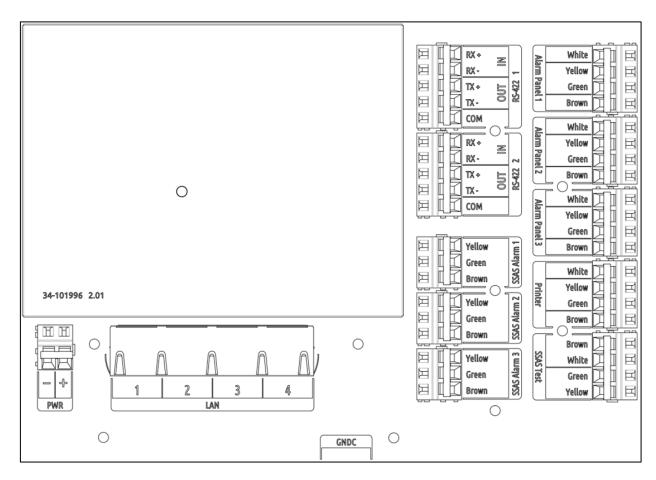
Figure 42: LT-3140S Interface Unit (with interface labels)
