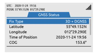
Figure 358: GNSS Receiver Integrity State
