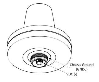
Figure 53: LT-3130 Antenna Unit (VDC(+), VDC(-), and GNDC)
