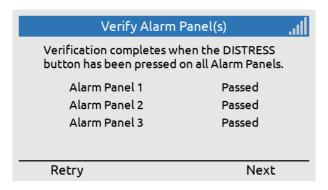
All Alarm Panels have passed the test, press Next to continue.
