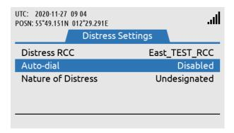
Auto-dial configured to Disabled (the LT-3100S GMDSS system will not automatically make a Distress Call to the RCC).
