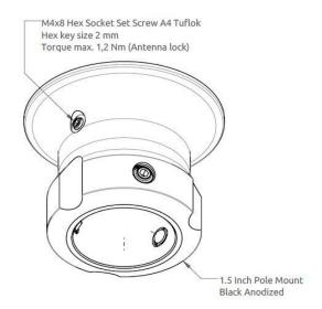
Figure 31: Pole Mount (1.5" pipe, Ø38.8 mm), Antenna Unit
