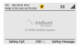
To go back to the default window press the 'Menu' button. By pressing the soft key 'MSI (1)' the user will be directed to the MSI window (1 unread MSI message).
