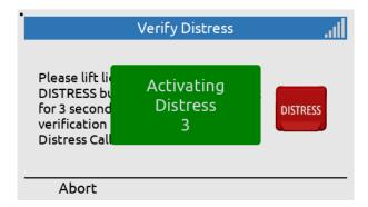
Lift the lid to the DISTRESS button and push the button for a minimum of three seconds (colored green to indicate test).
