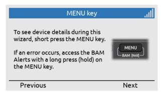
The MENU key can be used to access details (short press) during completion of the Installation Wizard.
