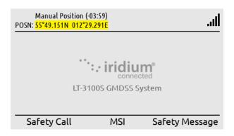
In the status bar the age of the Manual Position is shown. (-03:59) indicates that the position is three hours and 59 minutes old.
