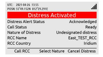
Distress Alert Status = Acknowledged (Distress Alert message has manually been ackknowledge by the RCC).
