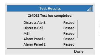
Upon finalizing the Terminal Test, the Test Results will be displayed.
