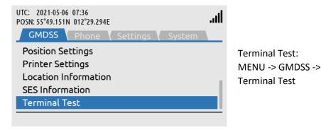
Figure 207: Terminal Test (1 of 18)
