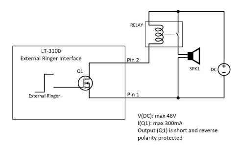
Figure 40: External I/O (external ringer diagram)
