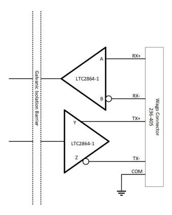
Figure 39: RS-422 Circuit Diagram for the LT-3110S CU
