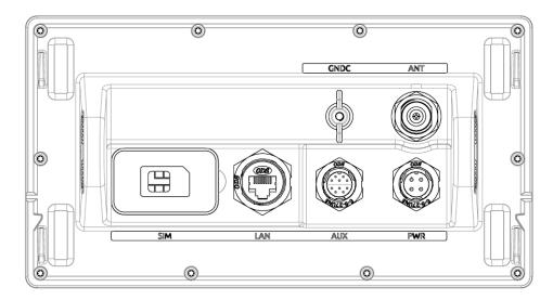
Figure 35: LT-3110S Control Unit (back view)
