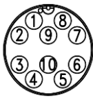
Figure 26: AUX connector pin out
