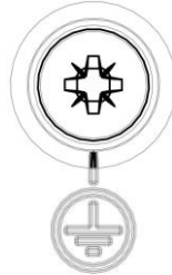
Figure 16: Chassis Ground (GNDC)
