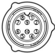
Figure 27: AUX cable pin out
