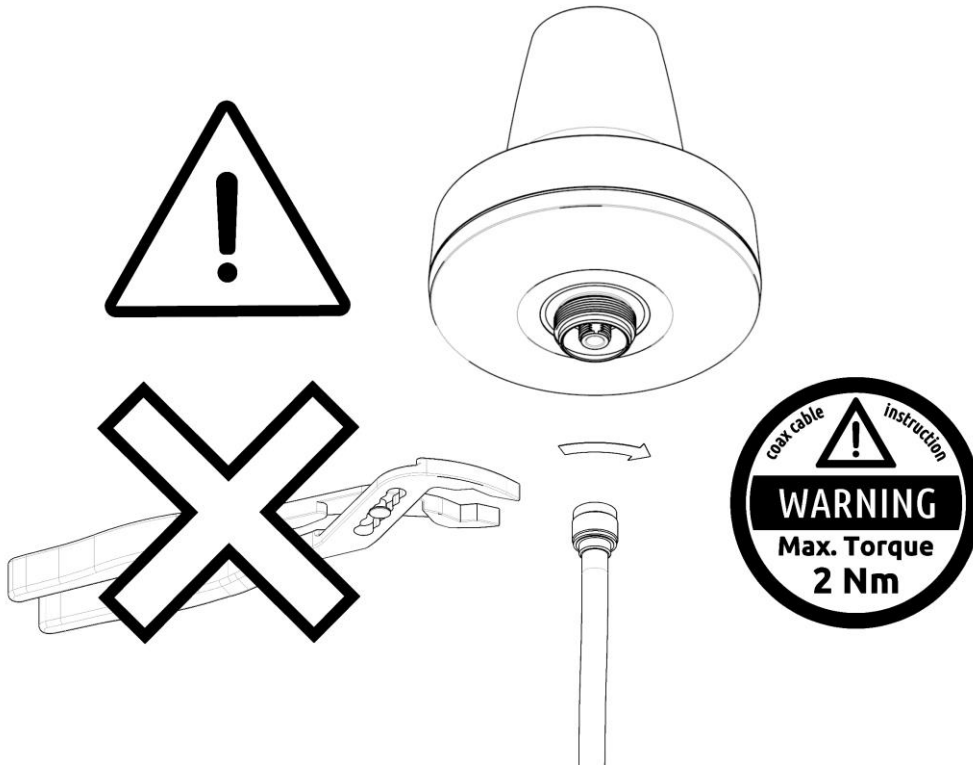
Figure 11: Connecting coaxial cable N-connector to the LT-4130 Antenna Unit
