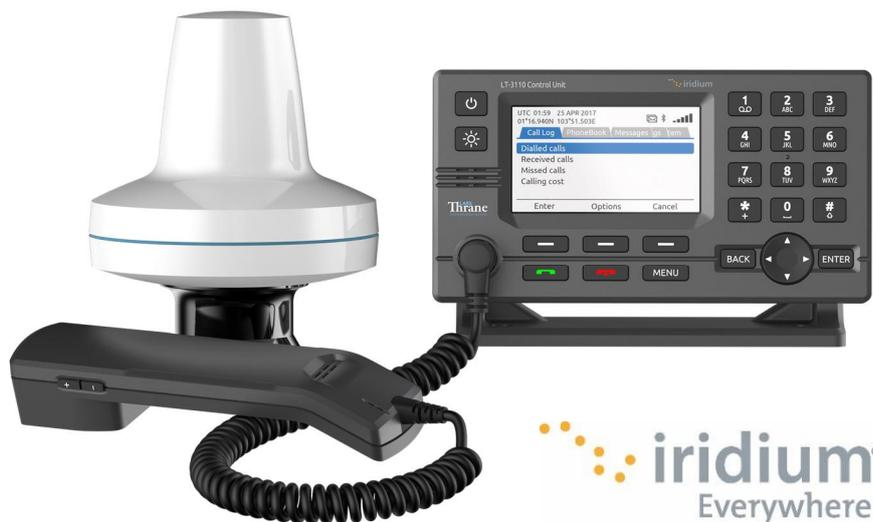
The LT-3100 system has voice and data capabilities with 100% global coverage via the Iridium satellites. The LT-3100 system consist of a control unit, handset-unit, and antenna unit. A single coaxial cable connects the control unit with the antenna unit. Up to 500 meters of separation between the units can be obtained, giving freedom to mount the antenna in the best possible location, with free line of sight to the satellites.
